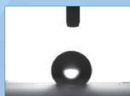
A-068 撥水品 接触角:130.2度 A-068 With treatment Contact angle: 130.2 degrees
